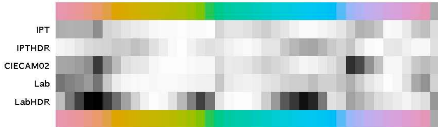
Fig. 6. Visualization of PCA analysis on the dimensionality of constant hue lines. Dark entries indicate that a significant amount of variation requires two dimensions to describe (an indication of hue nonlinearity).
