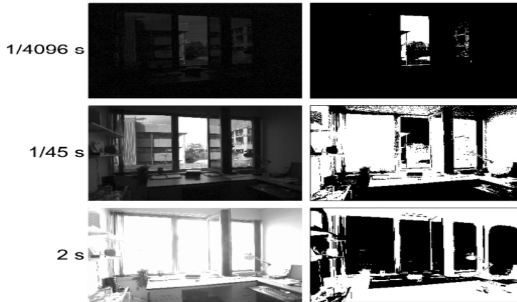
**Fig.7.** Using the feedback-based algorithm in Section IV-C, exposures at shutter speeds of 1/45s, and 1/4096s were captured (in that order). The resulting LDR images set is shown on the left of this figure. On the right of each LDR image is shown a map of the captured pixels for each image. Captured pixels are shown white, pixels that were either in saturation or below the system noise floor are shown in back.
