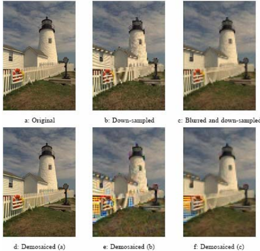
Fig. 2. HR image (a) captured by a 3-CCD camera is (b) down-sampled by a factor of four. In (c), the image in (a) is blurred by a Gaussian kernel before down-sampling by a factor of 4. The images in (a)–(c) are color-filtered and then demosaiced by the method of [16]. The results are shown in (d)–(f), respectively. (a) Original. (b) Down-sampled. (c) Blurred and down-sampled. (d) Demosaiced (a). (e) Demosaiced (b). (f) Demosaiced (c).
