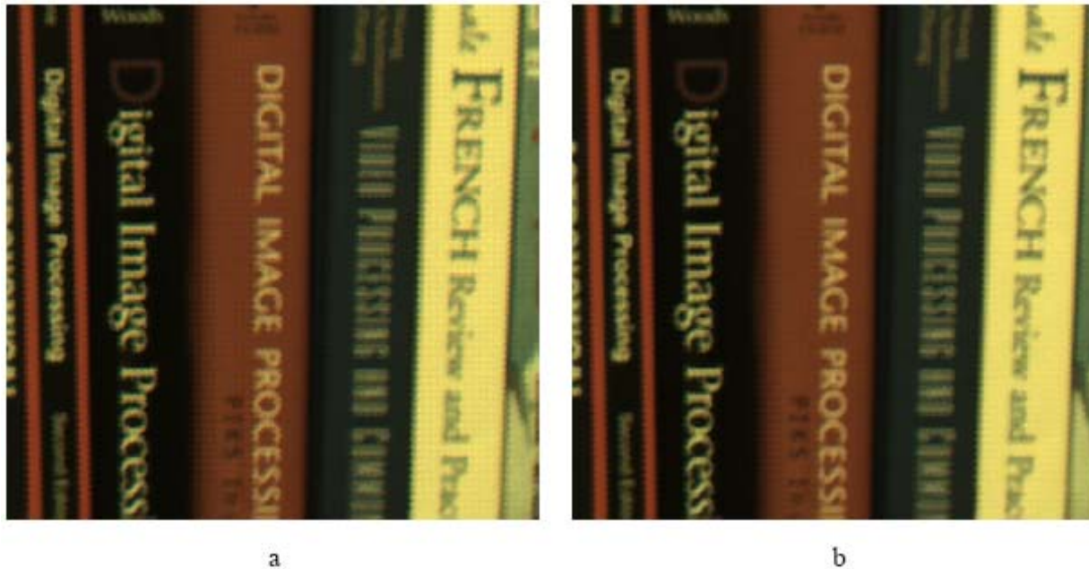
Fig. 14. Multiframe color super-resolution implemented on a real data sequence. The result of applying our method on the original un-demosaiced raw LR images (without using the inter color dependence term) is shown in (a). (b) Result of applying our method on the original un-demosaiced raw LR images.
