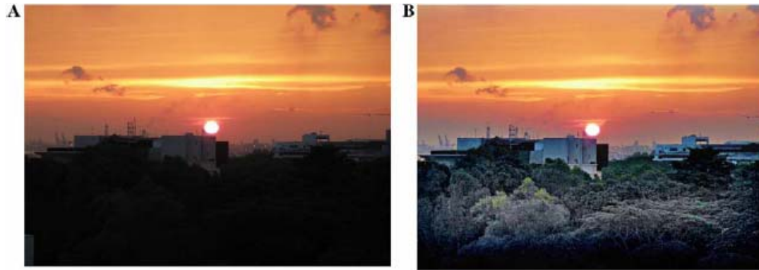
Fig.11. (A) Origin image captured by canon digital in auto-model sets CNI=0.7781 and CCI=21.2713. (B) HCCIEE algorithm enhanced color image CNI=0.9732 and CCI=19.6171.
