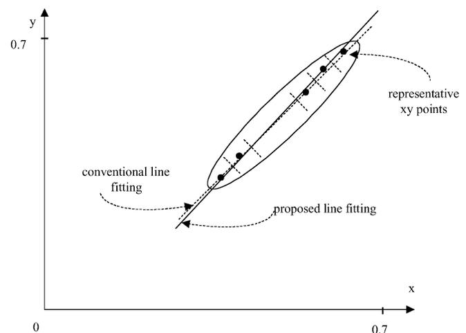
**Figure 4.** 2-D representation of proposed extraction of line parameters.
